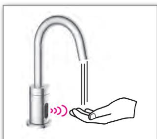
The tap is fitted with a sensor which activates in the presence of an object in front of it.
